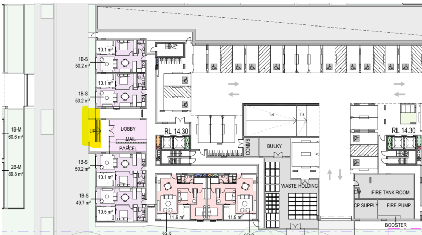
Figure 3 – Extract of Level 04 illustrating location of stairs (highlighted in yellow) into the lobby of the Social housing building.
