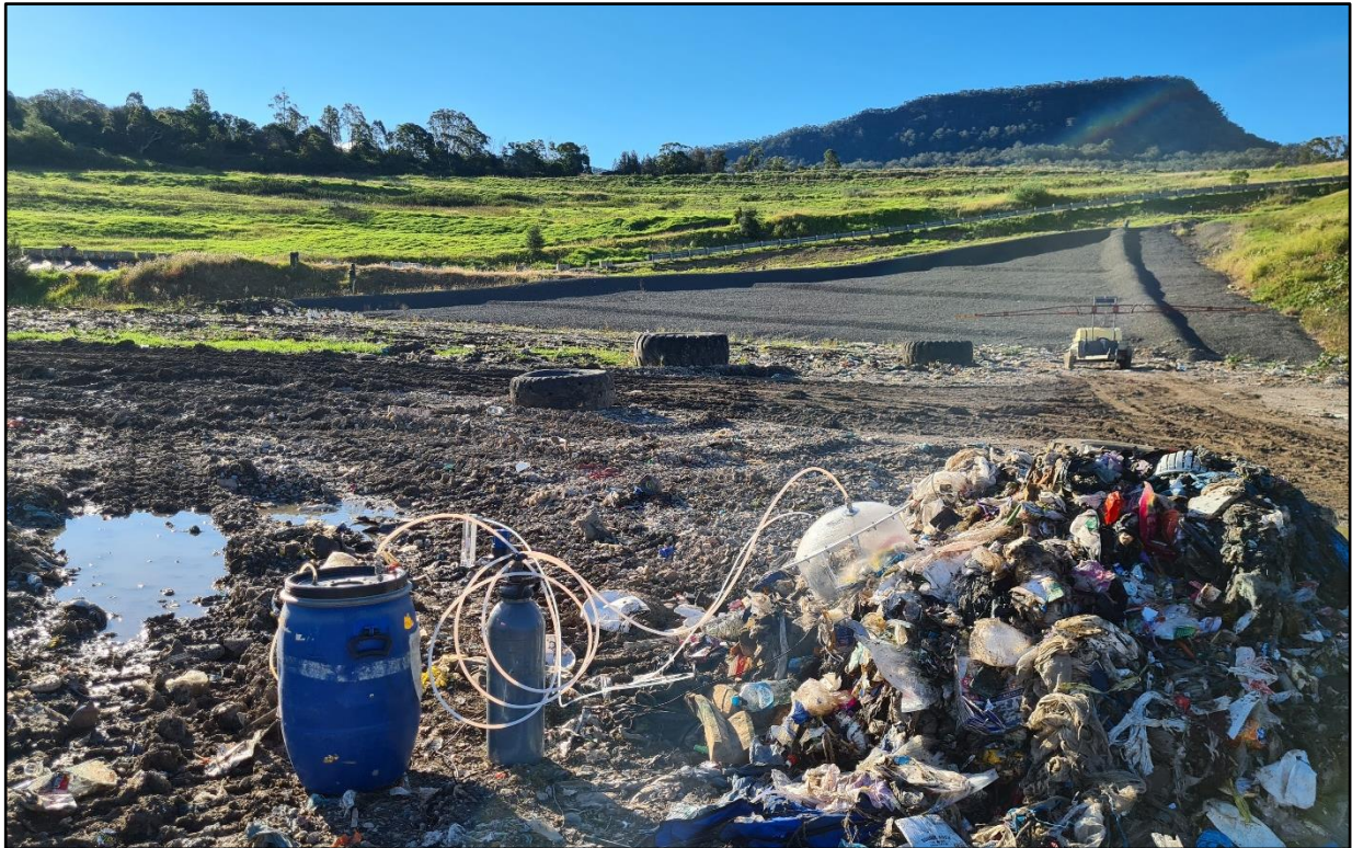
Photo 2.5 – An example of IFH sampling on the active tipping face material dated 10 May 2021
