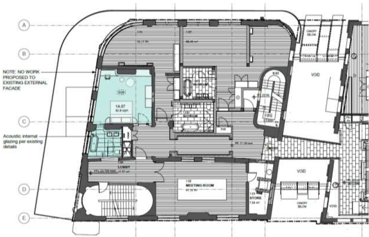
Figure 5 - Proposed Room 1.07 in former Level 1 Manager's Office
