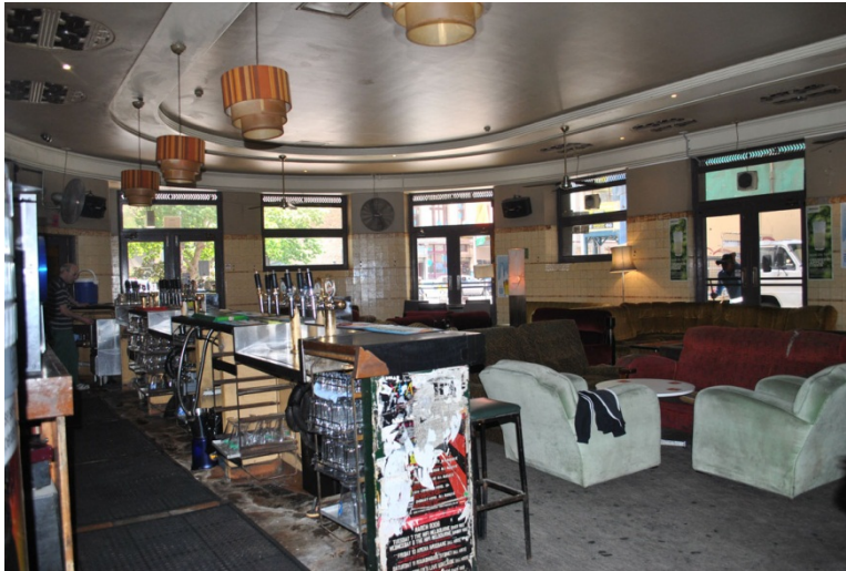
Figure 80. The main Public Bar is a very good example of its type. The space was originally dominated by a long elliptical counter in the centre of the room (which was intended to maximise serving efficiency), the curve of which was reflected in the detailing still seen in the ceiling above the space. The use of the streamlined, curving element as the underlying design theme is typical of Art Deco and is used throughout the hotel. The curve of the exterior wall is reflected in the interior, creating an intimate sense of space.
