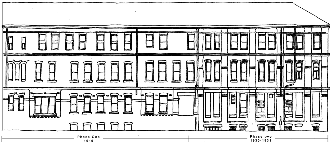
Figure 26. Eastern elevation of the Administration Building showing the major phases in its development. The upper level was added at the same time as the northern extension but noticeably less care was given to ensuring that the fenestration patterns are consistent with those on the lower levels on this side of the building, although the overall rhythms and disciplined character of the facade are retained.
