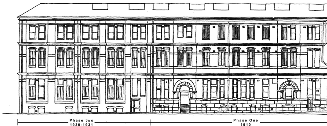
Figure 25. The main facade of the Administration Building faces what was originally the main brewery driveway and is now to be known as Carlton Street. The main phases of the development of the building are shown.
