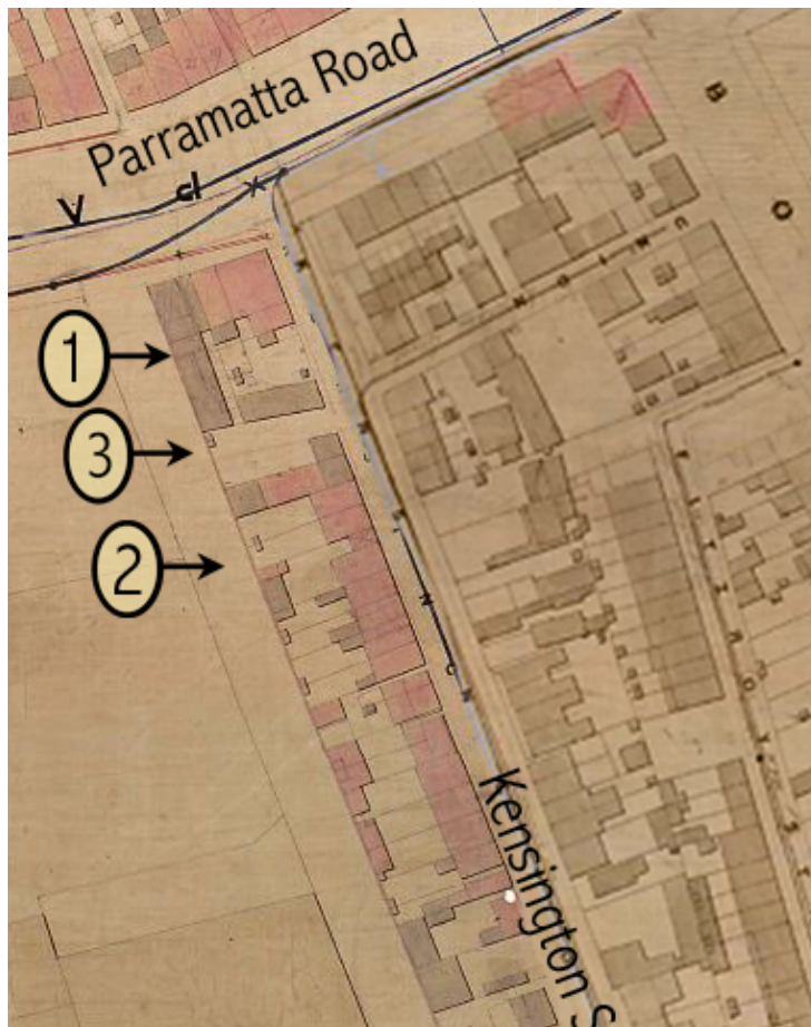
Figure 6. Composite extract from the 1865 Trigonometric Survey of Sydney showing the pattern of development along Kensington Street. Parramatta Road has not been widened, with three separate buildings shown between Kensington Street and the Brewery driveway (1). The rookery seen in Figure 6 was no longer occupied, but the footprint suggests that the structures may have remained on the site. The western side of Kensington Street (now mostly occupied by the Administration Building) was lined by modest terrace and small industrial buildings (2). The location of the service lane between the two buildings is suggested on this plan by the spacing of the buildings (3), but no evidence was found that it was reserved for a lane at this time. (Trigonometrical Survey of Sydney 1855-1865. Sheets U1 (west side of Kensington Street) and S2 (east side). Sydney City Council Archives.)
