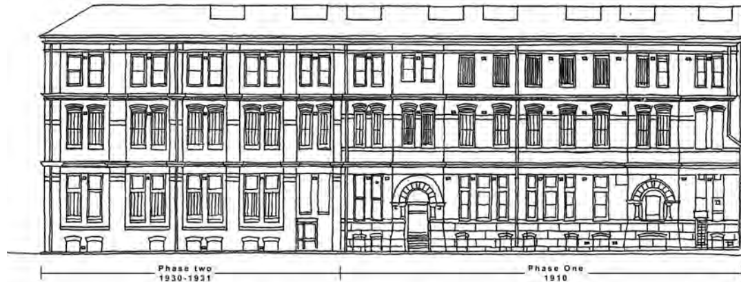
Figure 4: The main facade of the Administration Building faces what was originally the main brewery driveway and is now to be known as Carlton Street. The main phases of the development of the building are shown.
