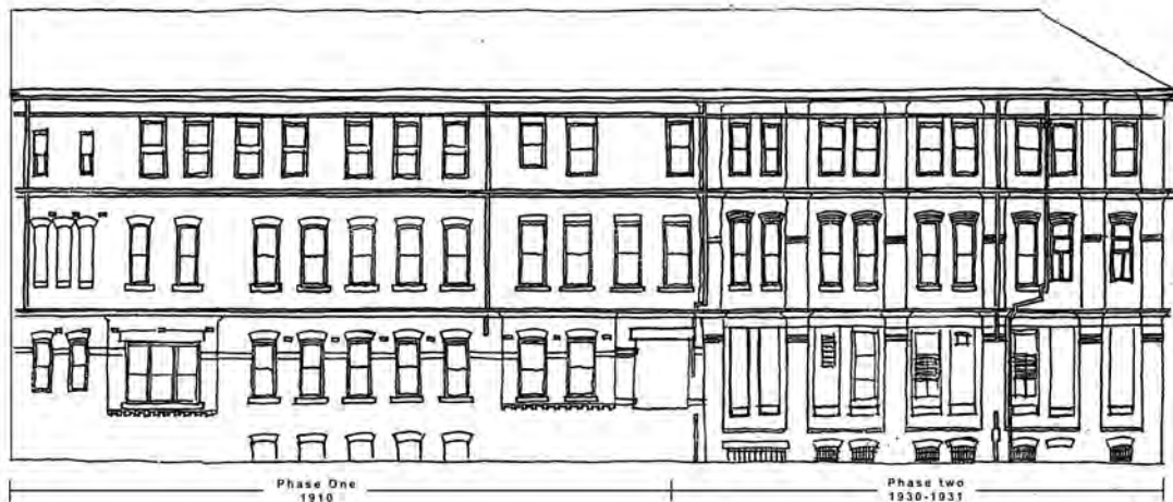
Figure 5: Eastern elevation of the Administration Building showing the major phases in its development. The upper level was added at the same time as the northern extension but noticeably less care was given to ensuring that the fenestration patterns are consistent with those on the lower levels on this side of the building, although the overall rhythms and disciplined character of the facade are retained.
