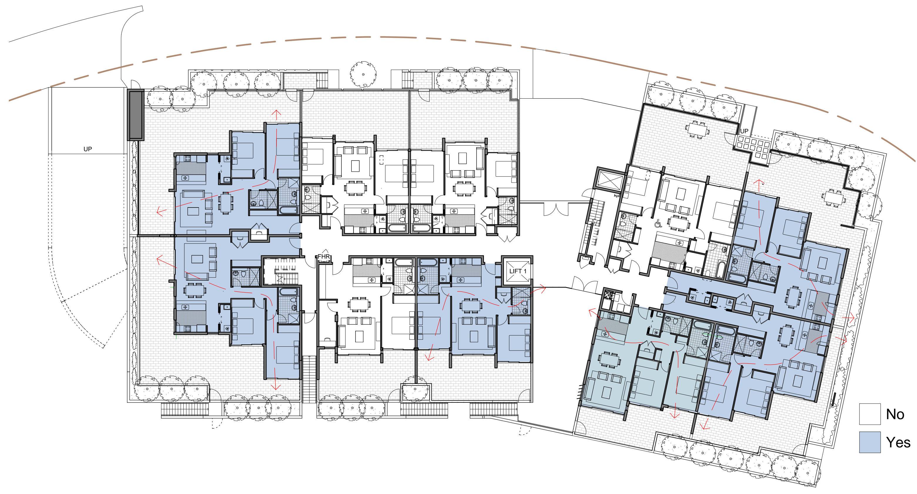
1 CROSS VENTILATION (GROUND LEVEL) 1 : 200
