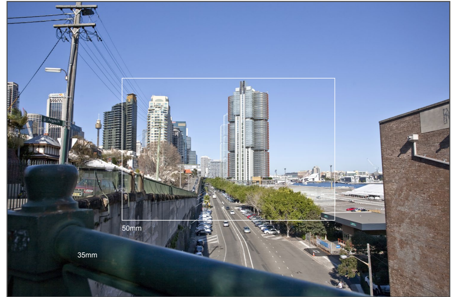
Image showing proposed building montaged into existing photograph & crop marks for longer lenses sizes.
