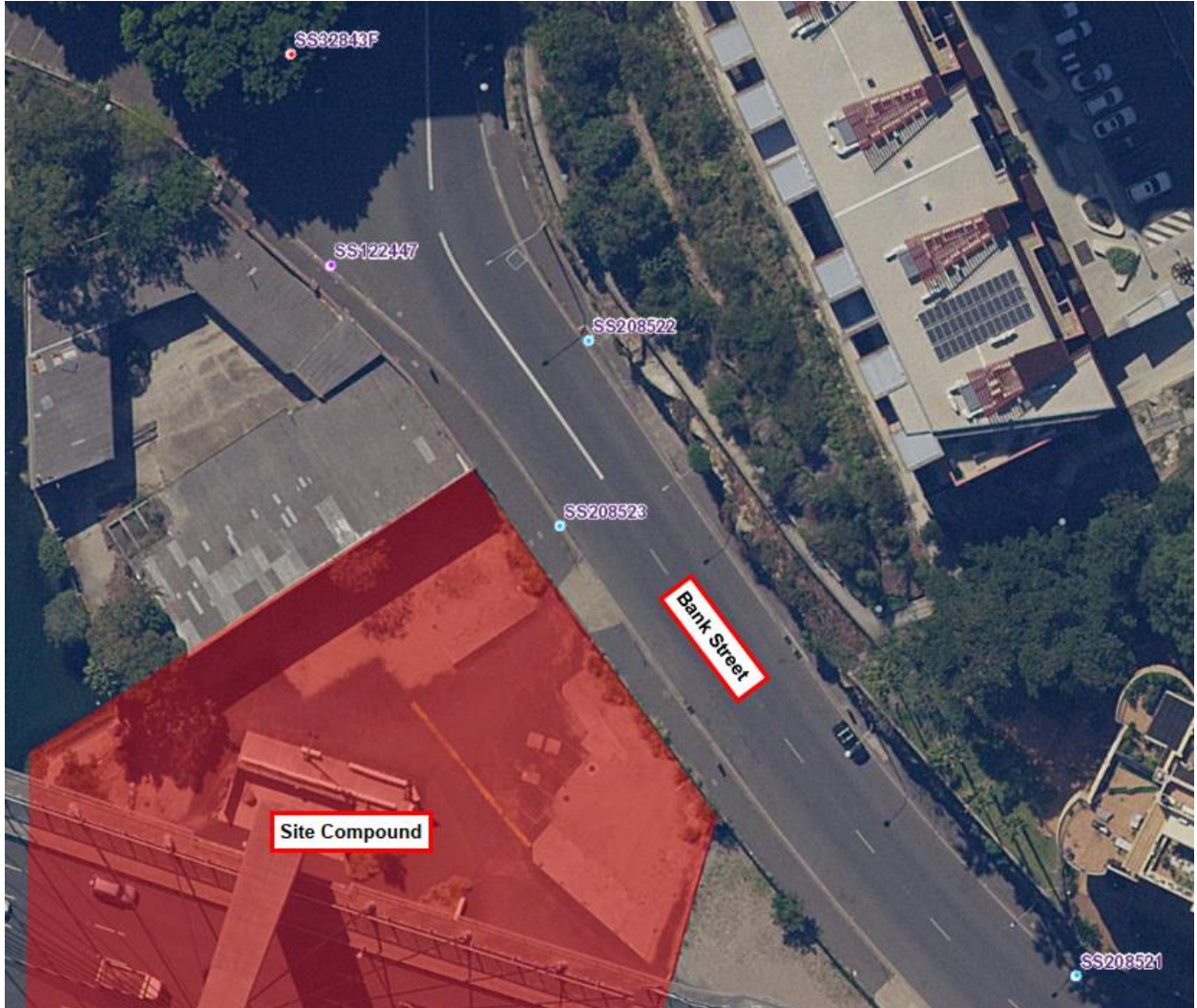
Figure 2 - State Survey Mark Locations
