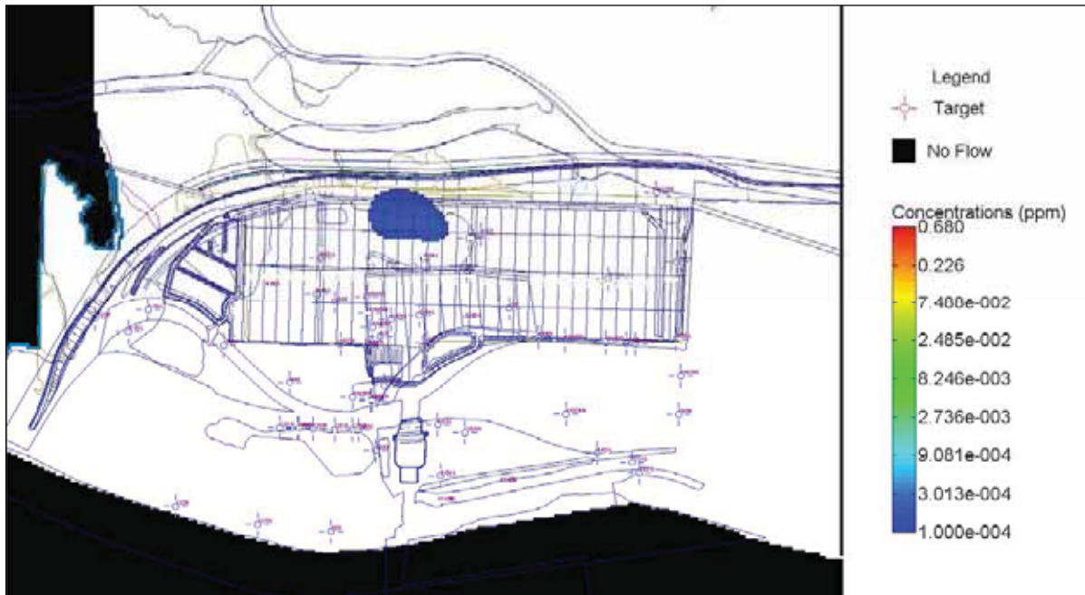
Figure 23: Lead concentration Contours in the Estuarine Aquifer 100 years After Capping of Site, with Decay in the PRB Gates due to Chemical Reactions, Dispersion and Sorption
