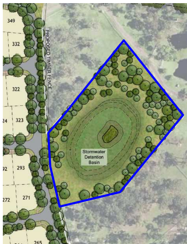
Figure 10. Location of stormwater detention basin (known as Dam 2) on the residual lot to function as a wetland. The proposed easement for drainage is in blue.
