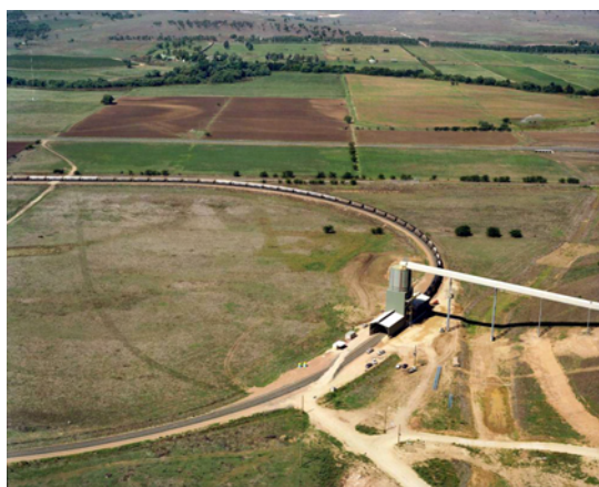
A rail loop for coal loading designed to avoid productive alluvial farm lands. Photo: D Barnes.
