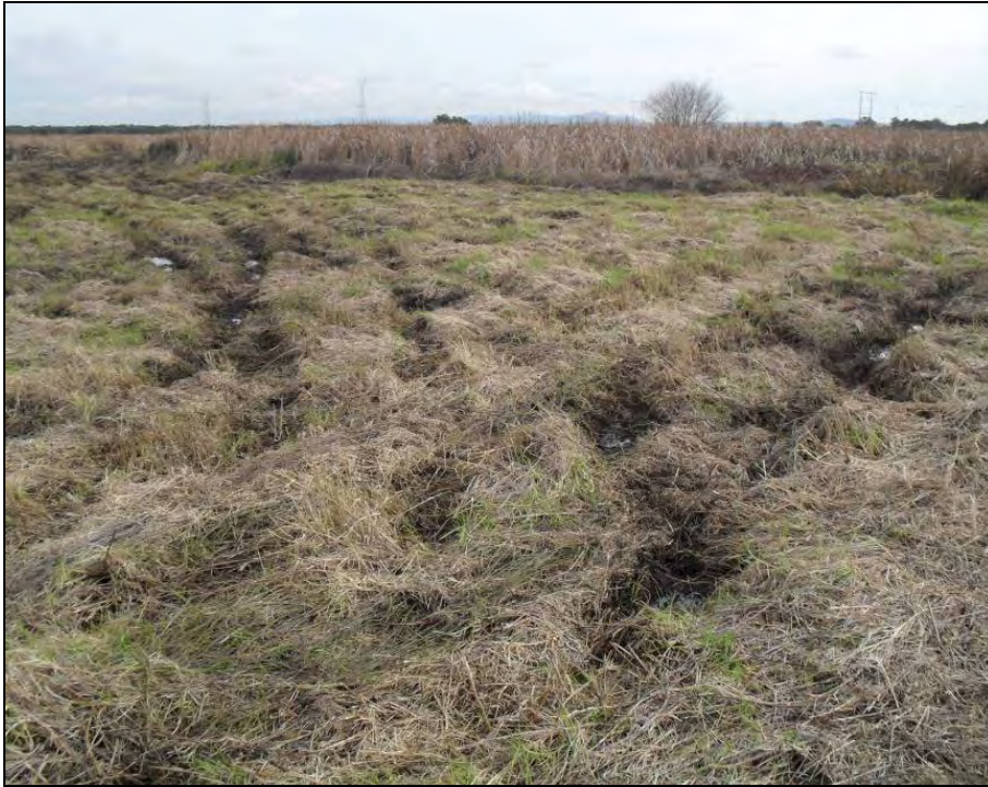
Photo 11 – Low-lying saturated surface soils in slashed paddock with rutting evident from tractor (looking south west)
