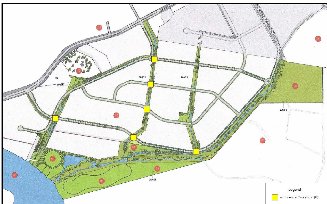
Figure 16 - Fish Friendly Crossings Post Development.
