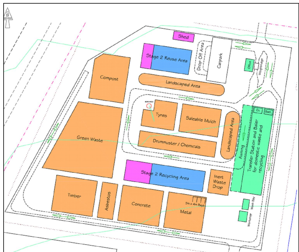
Figure 5-3 Site Layout (Operational Area)
