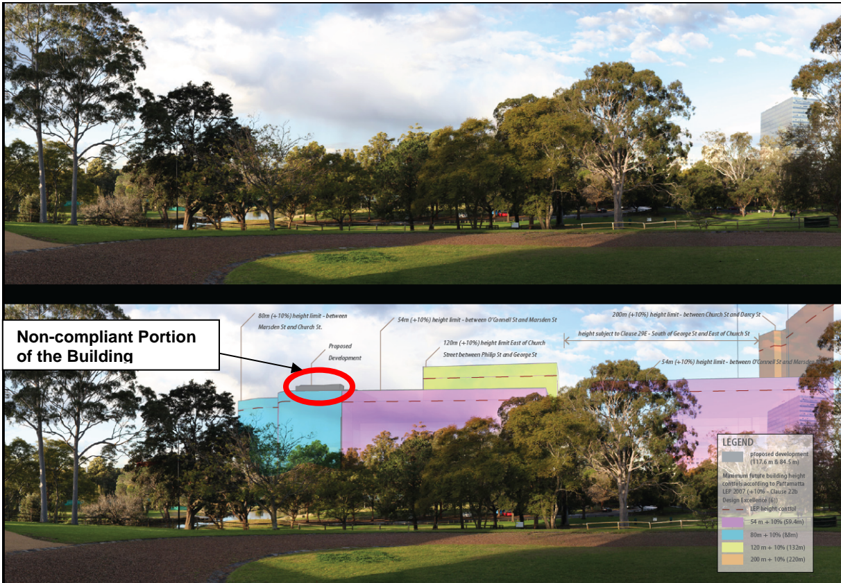
Figure 10: Comparison of Compliant Building Envelopes 1 and the Non-Compliant Portion of the Project.
