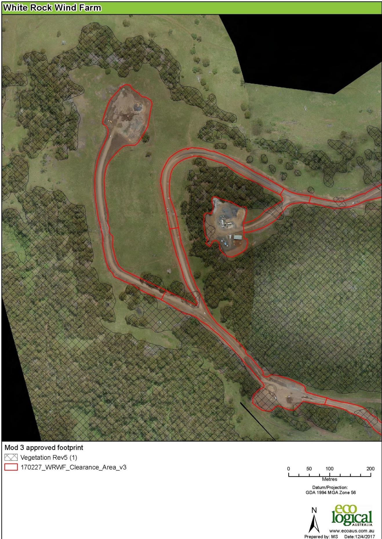
Figure 2: Extent of disturbance associated with construction to 27 February 2017
