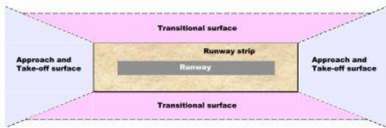
Figure 2 Obstacle Limitation Surfaces
