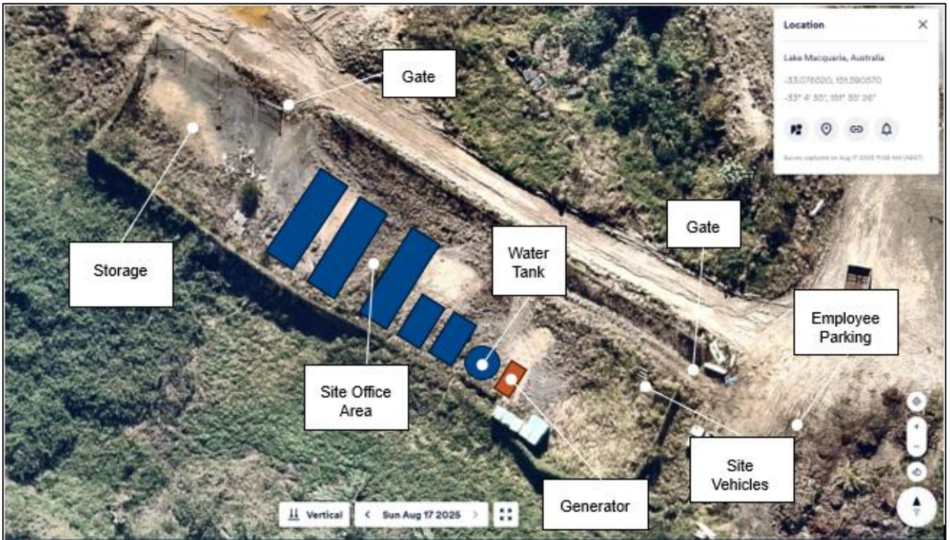
FIGURE 1-5 SITE COMPOUND LAYOUT
