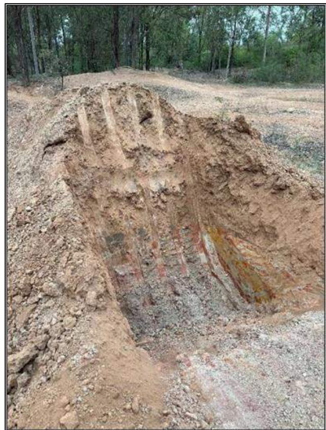
Figure 5-4 Typical existing overburden fill pile overlying in-situ residual soils and weathered materials ('TPCL02') - looking south
