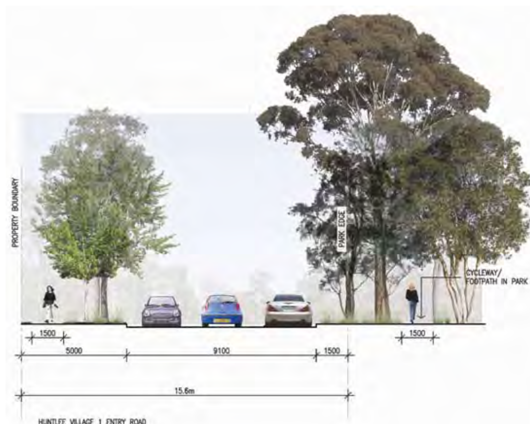
Figure 16 – Stage 1 Wine Country Drive Road Carriageway and Reserve Widths Source: Hassell
