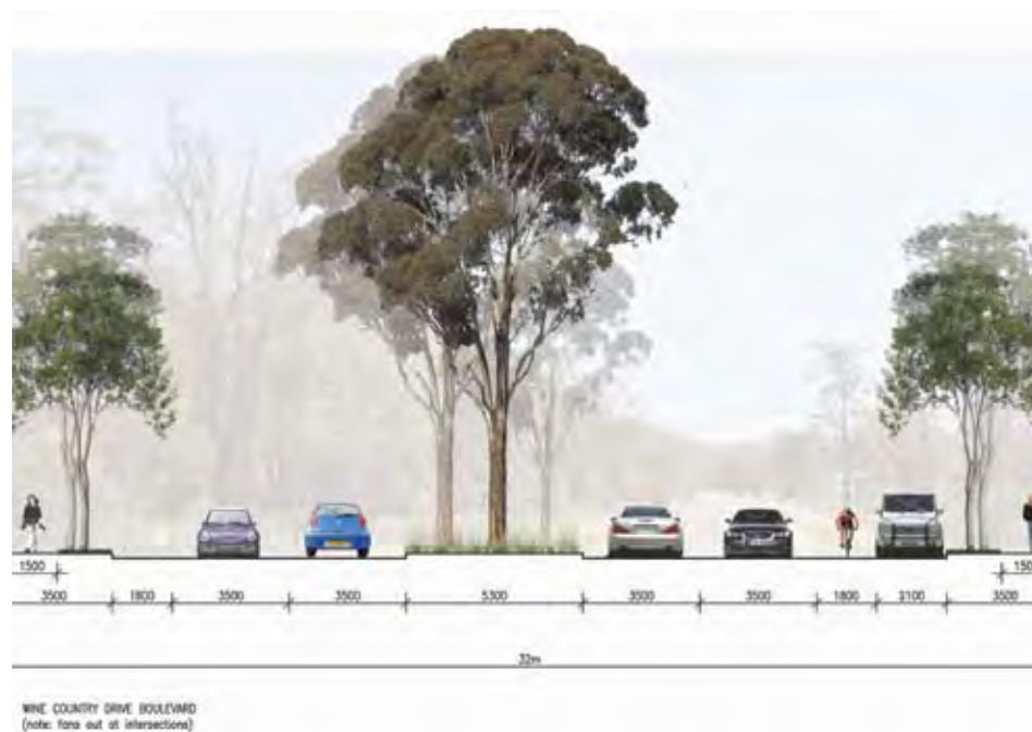
Figure 16 – Stage 1 Wine Country Drive Road Carriageway and Reserve Widths Source: Hassell
