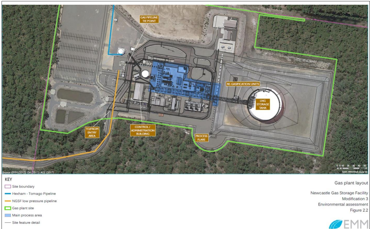
Figure 3: Gas plant layout
