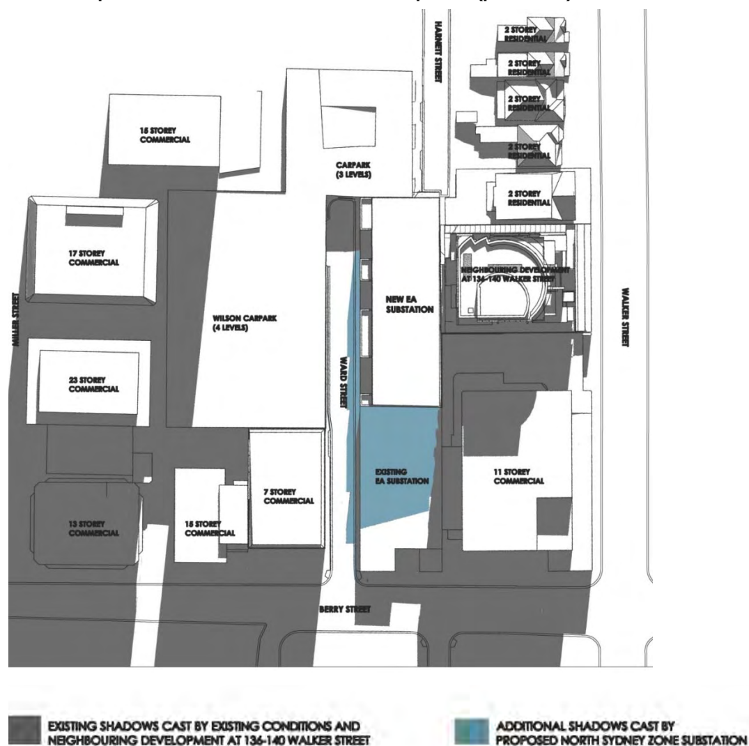
Figure 9-16 – Shadow Diagram for the Winter Solstice at 11:30am showing shadow affects on the Proposed 136-140 Walker Street Development (plan view)
