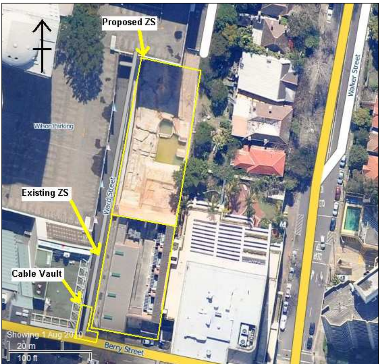
Figure 1.1 – Aerial View of Existing ZS and Proposed Works Location
