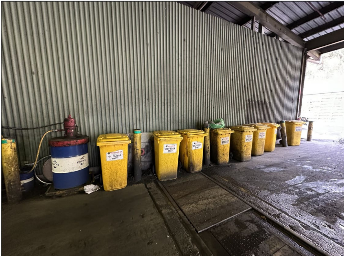
Photograph 07 – Waste segregation and Spill kits.
