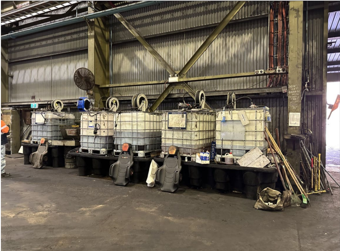
Photograph 05 – Bunded hydrocarbons in the Workshop meeting AS1940.
