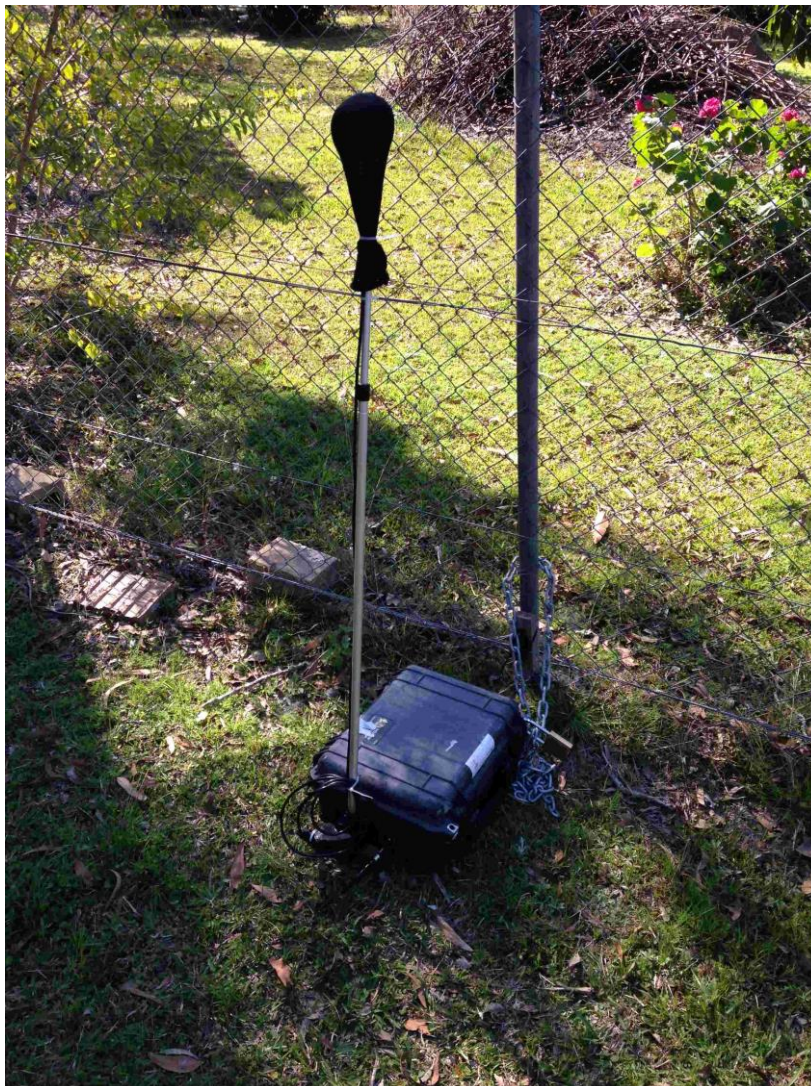
Figure 2 - Example unattended noise logger setup
