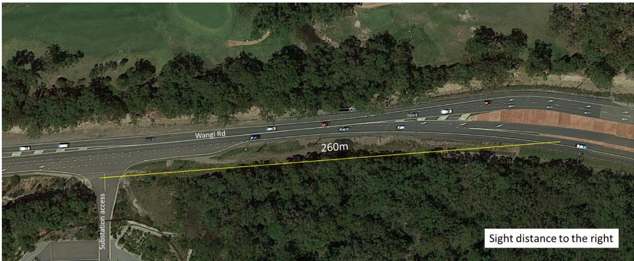
**Figure 4.5** Sight distance from the substation access intersection onto Wangi Road
