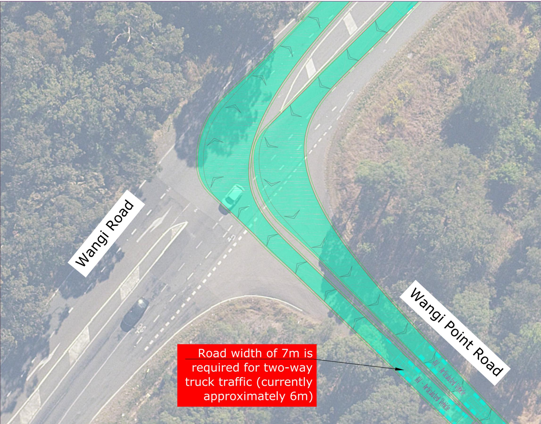
Road width of 7m is required for two-way truck traffic (currently approximately 6m)
