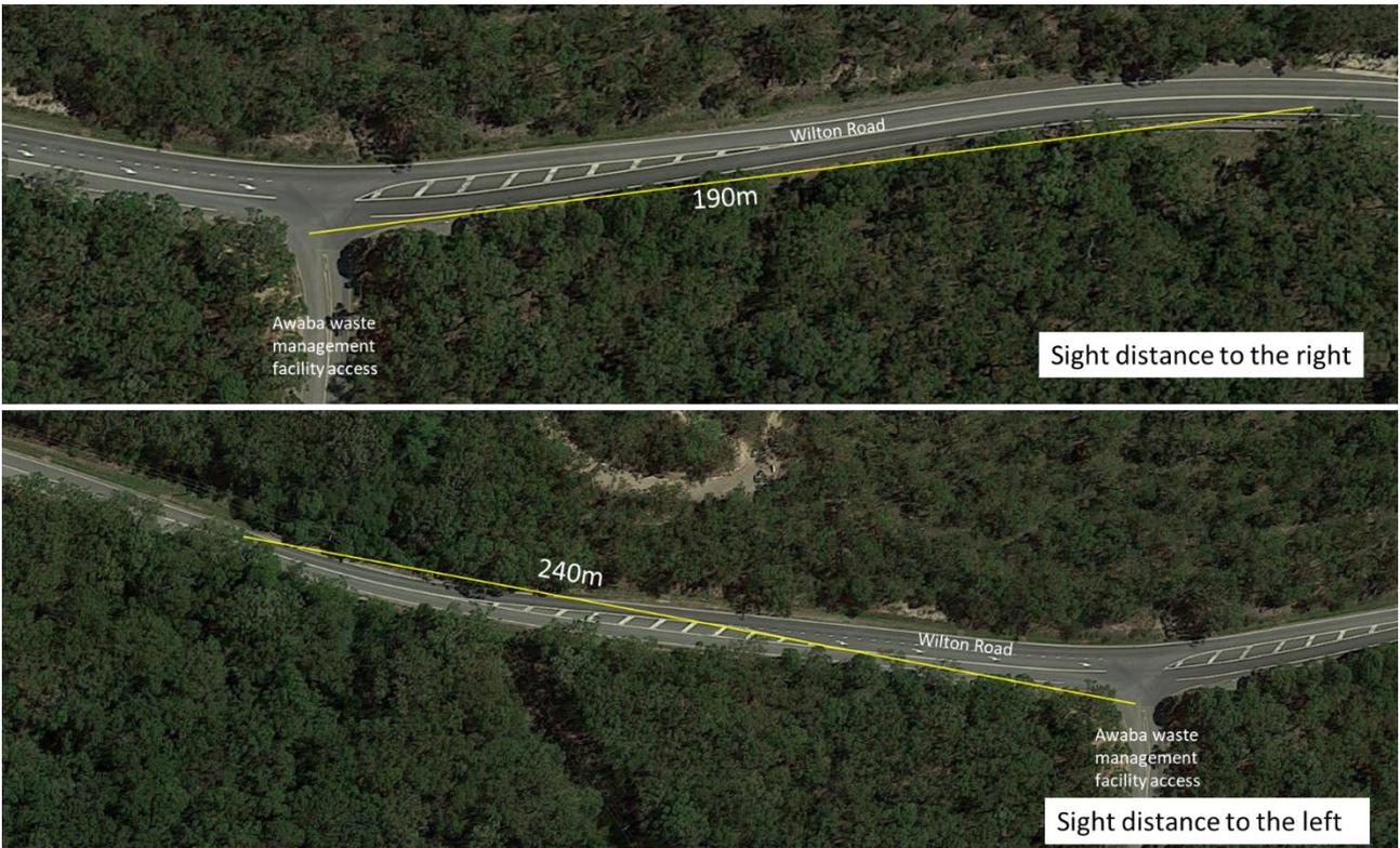
**Figure 4.6** Sight distance from the Awaba Landfill and Waste Transfer Station access intersection onto Wilton Road
