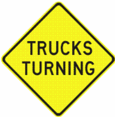
Figure 4.8: Trucks Turning Warning Signage – W5-205
