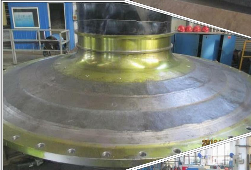
Plate 7: Primary Ball Mill feed head-drilling completed
