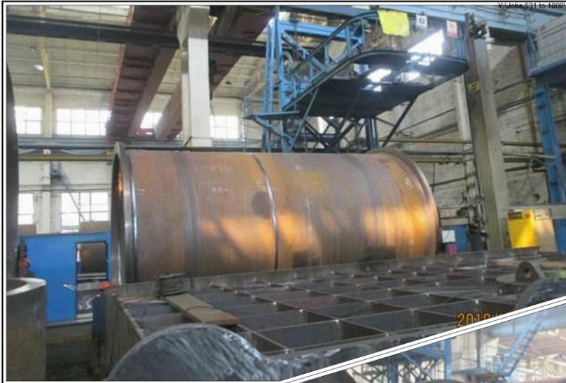
Plate 5: Primary Ball Mill shell welding in progress
