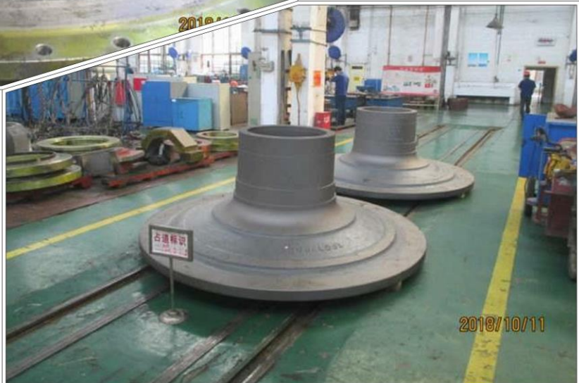
Plate 8: Regrind Mill feed head and discharge head blasting and primer completed
