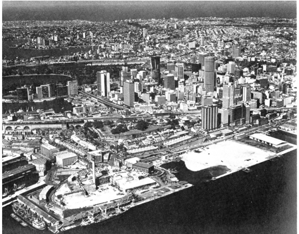
Fig. 2.16: 1971 image of Millers Point indicating the reclamation of the site for containerisation, the construction of the Harbour Control Tower and the further cutting away of sandstone for the creation of flat dock area
