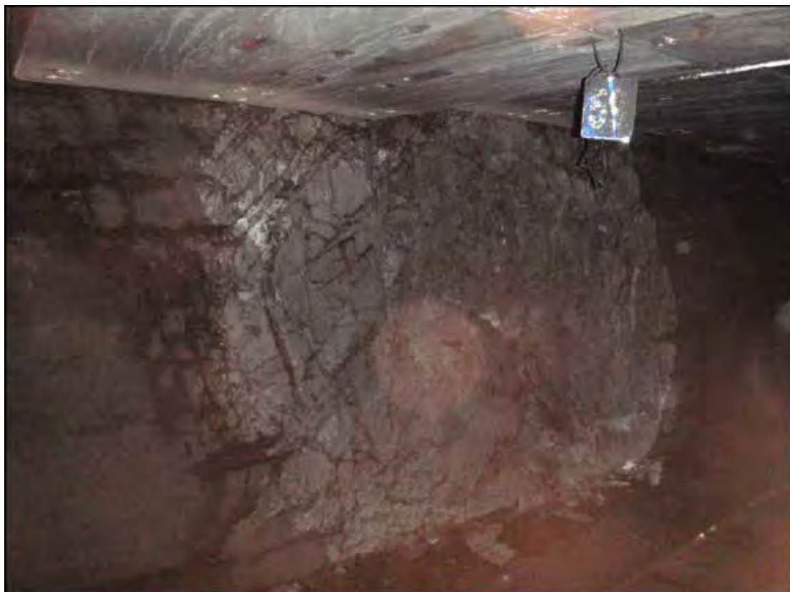
Figure 9: Dyke D8 exposed in the face of Longwall 5 on 21 June 2013. (Note this dyke was intersected at a shallow angle so the dyke appears thicker than it is).
