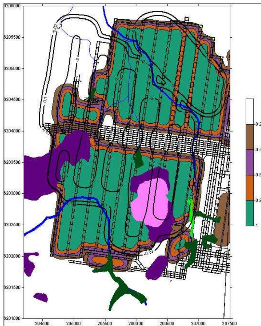
Figure 55 Compilation of subsidence and surface aspects of Area 3 in Wongawilli West (shaded contours – Bulli Seam subsidence, black line – 20mm and 100mm of Wongawilli subsidence, green areas – swamps, purple/pink – transitional forests)
