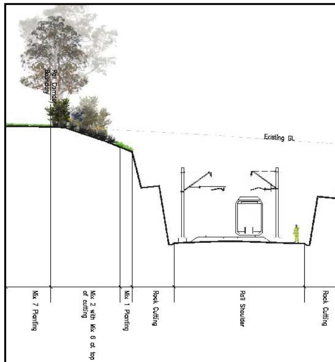
(b) - Typical cutting, shrub and groundcover on cut, and scattered trees on natural ground at top of cut Figure 4.5: TYPICAL SECTIONS - CUTTING
