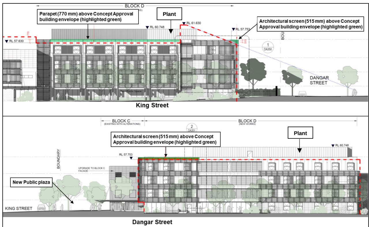
Figure 8: Modified King Street (top) and Dangar Street (bottom) elevations and the the location of height encroachments (Base source: the modification application)
