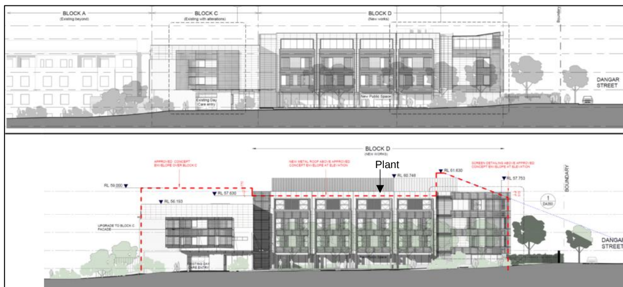
Figure 6: Approved (top) and proposed (bottom) King Street elevation, Concept Approval building edge maximum height (required by FEAR 8) shown as red dashed line (Source: MP10_0044 and Proponent's application)
