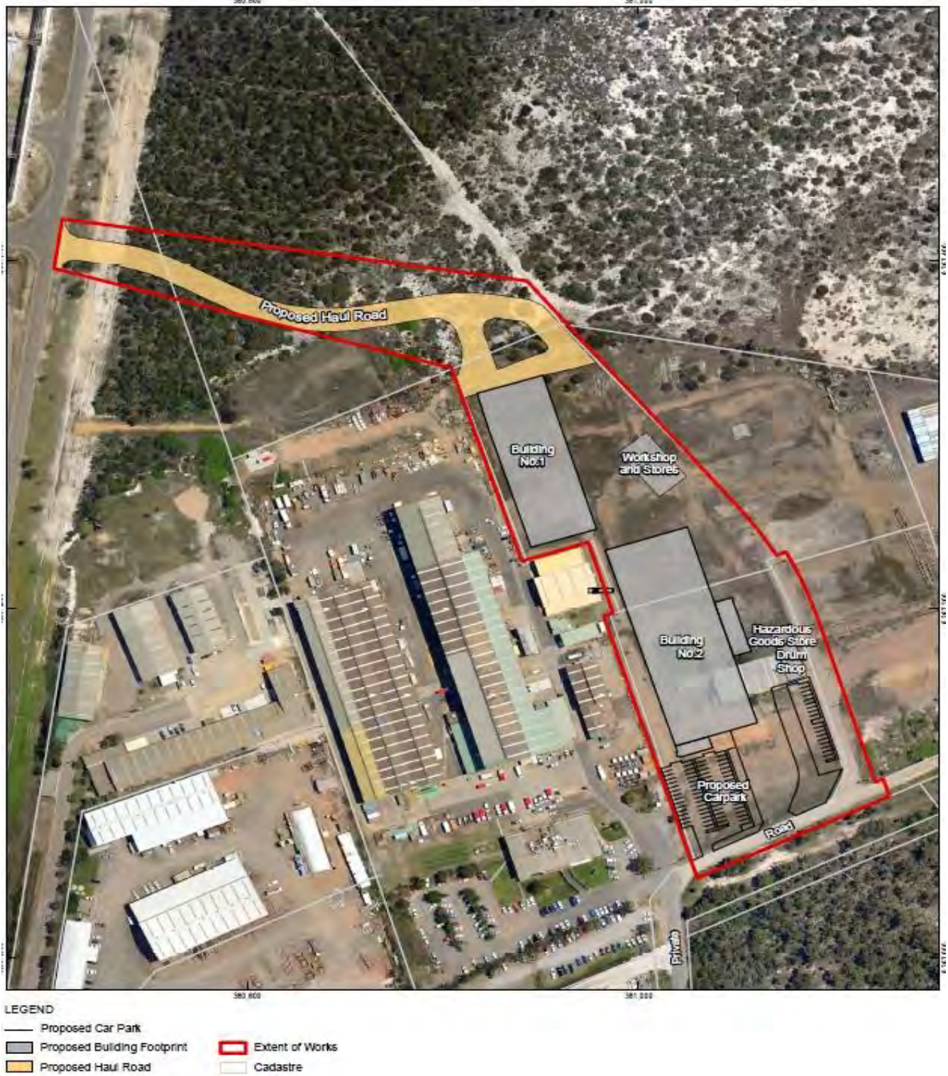
Figure E.3 Layout of key project components
