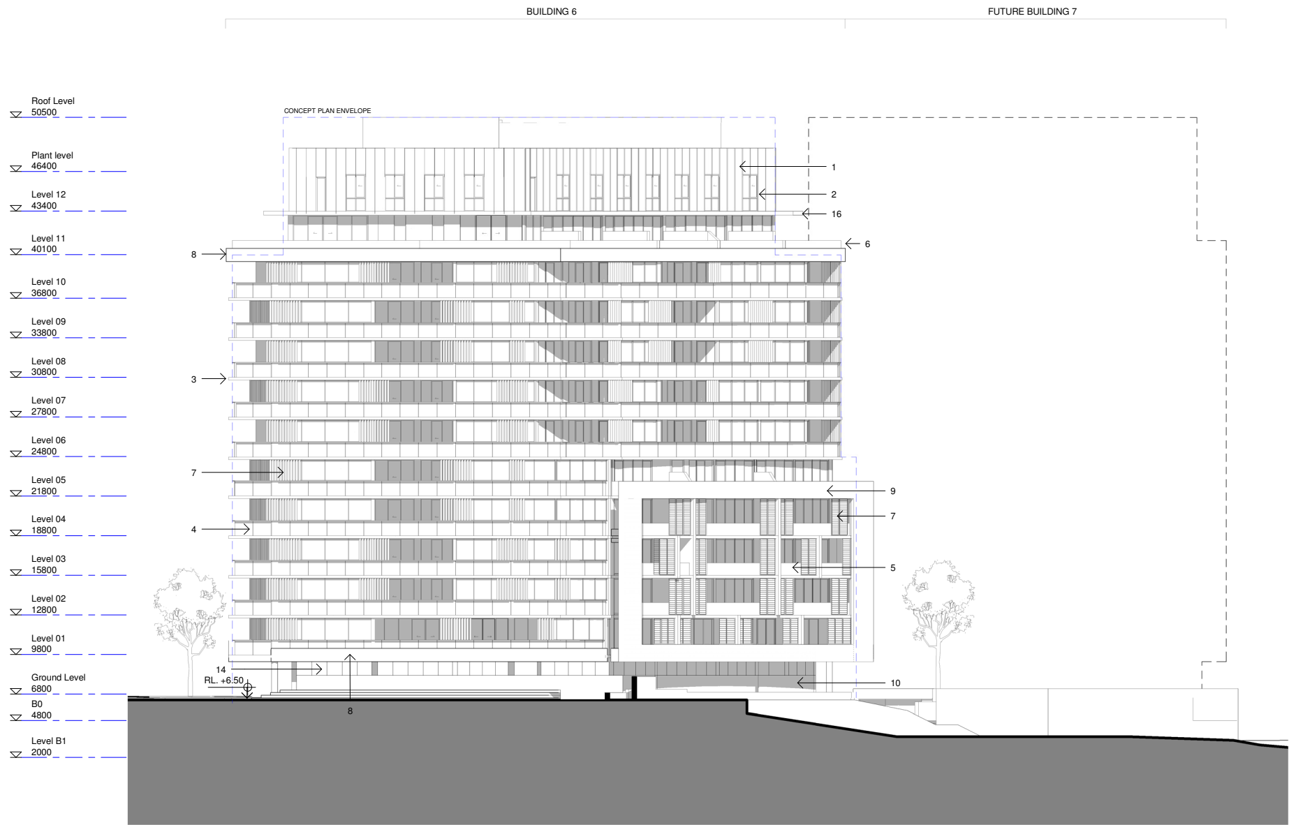
1 DA8.04 Section D - Building 6 South West Elevation 1 : 200
