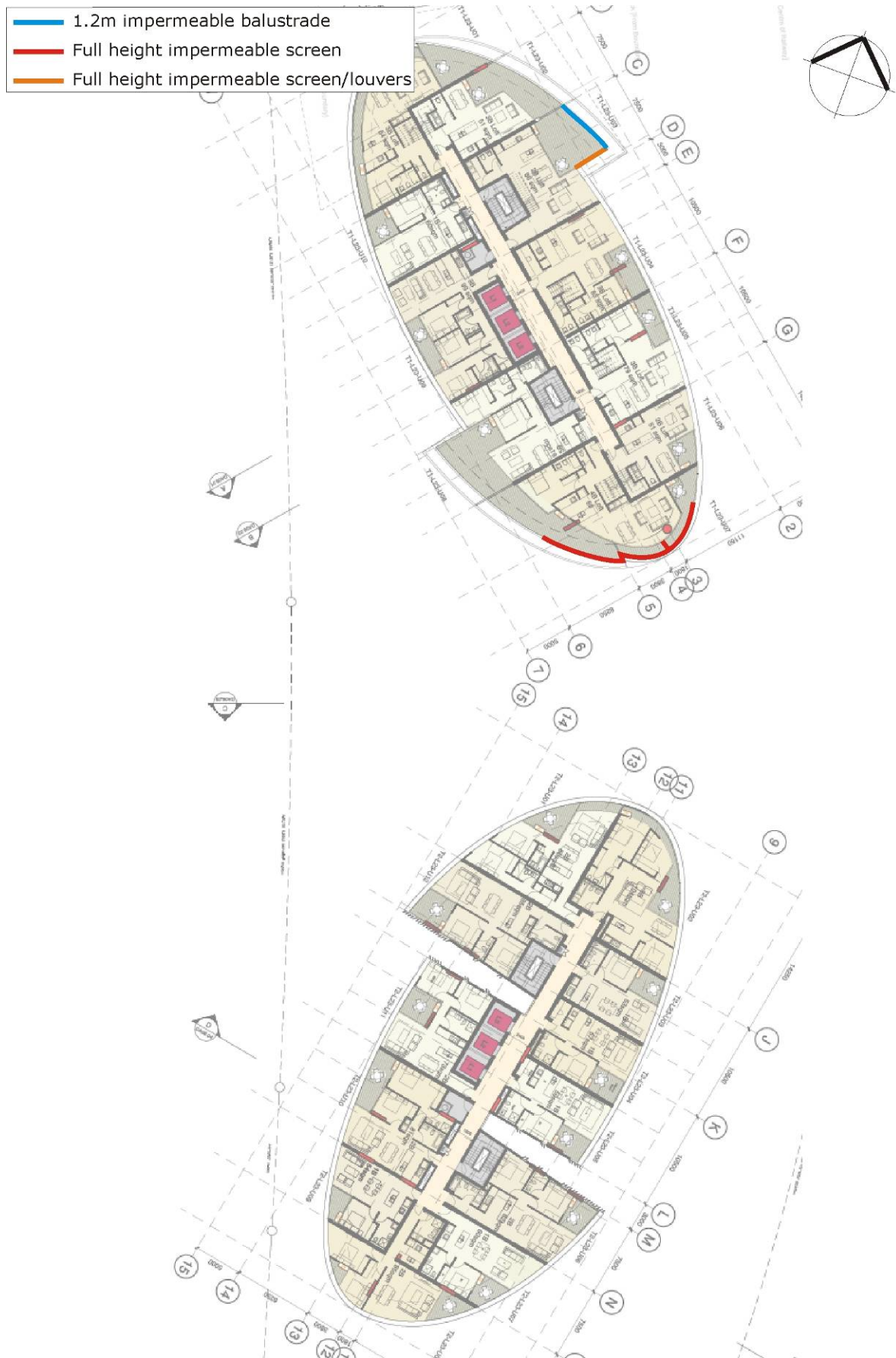
Figure 9e: Recommended Treatments for Level 23
