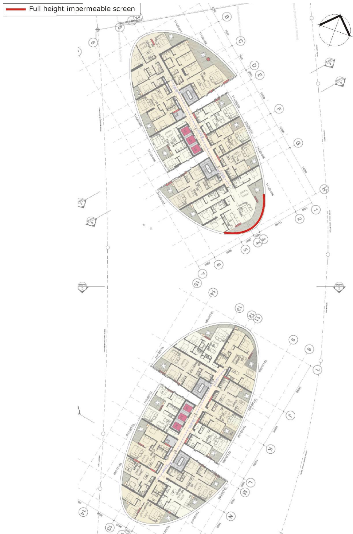
Figure 9d: Recommended Treatments for Level 22
