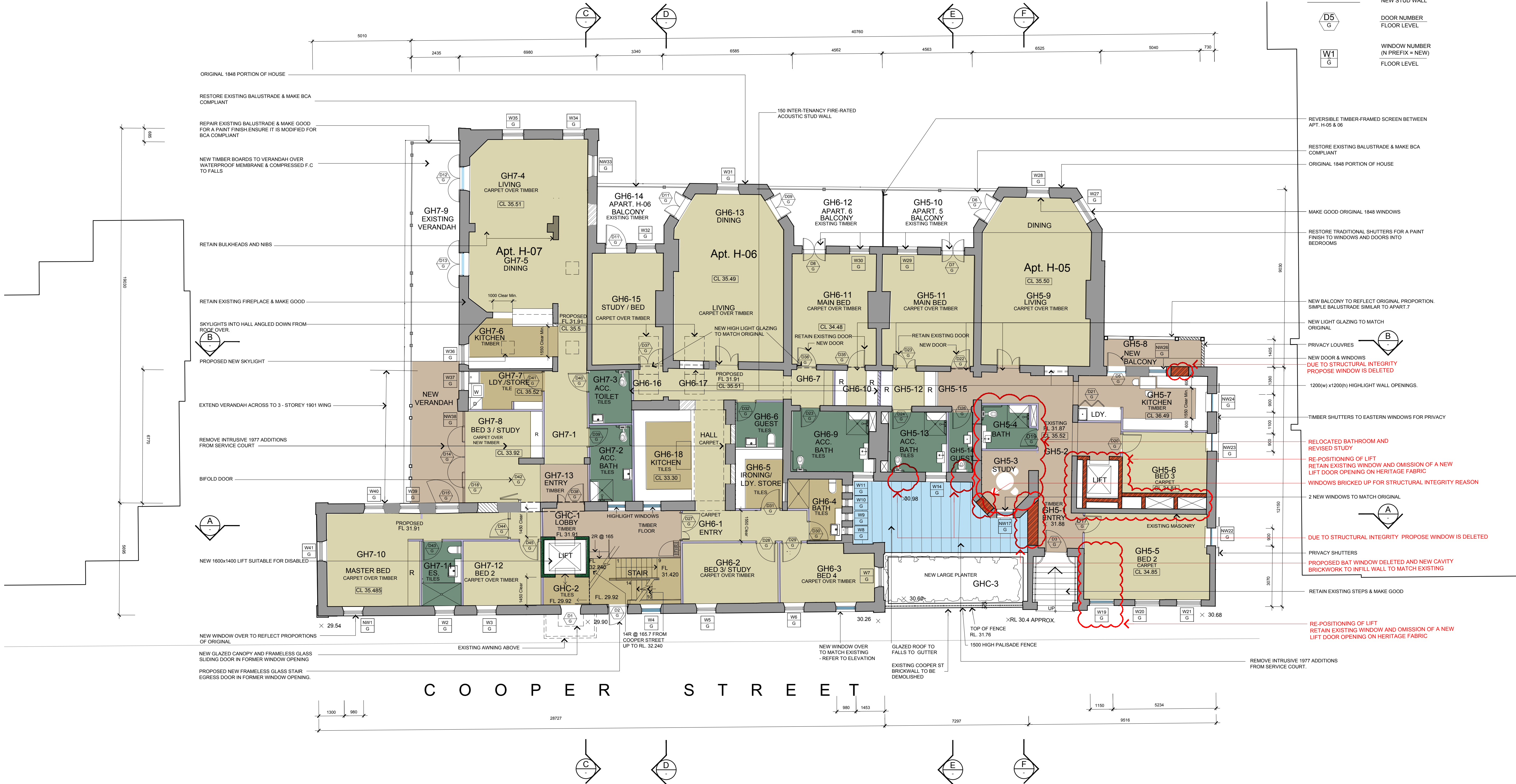
01 PROPOSED GROUND FLOOR PLAN : RL 31.88, RL 31.91 (OPTION A - DEMOLISH - NORTH - EAST CORNER) TO AS 4299 1:100@A1
