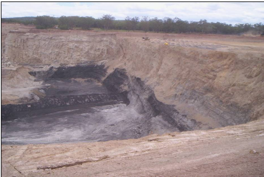
Photo 1 - Northern face showing shear zone with Belmont Seam to the west and Glenroc Seams to the east
