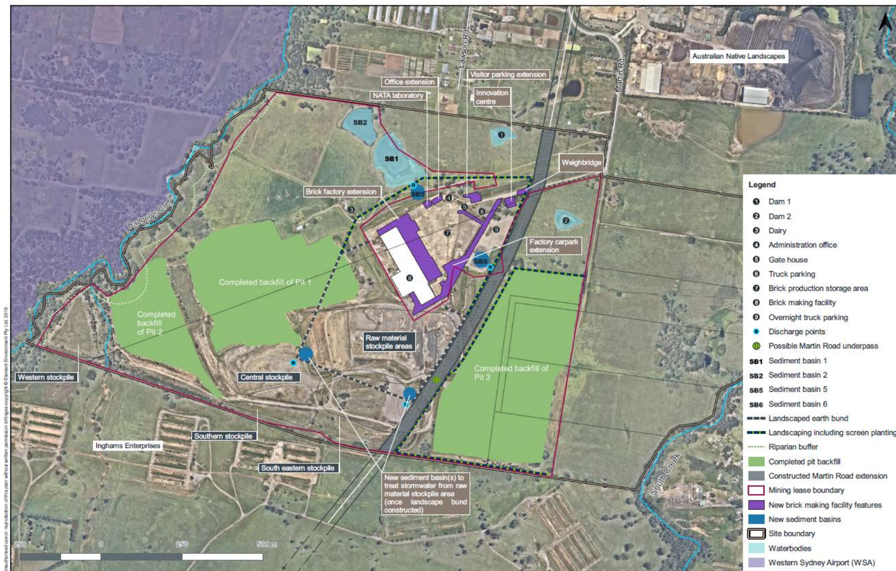
Figure 5: Phase 4 Project Layout
