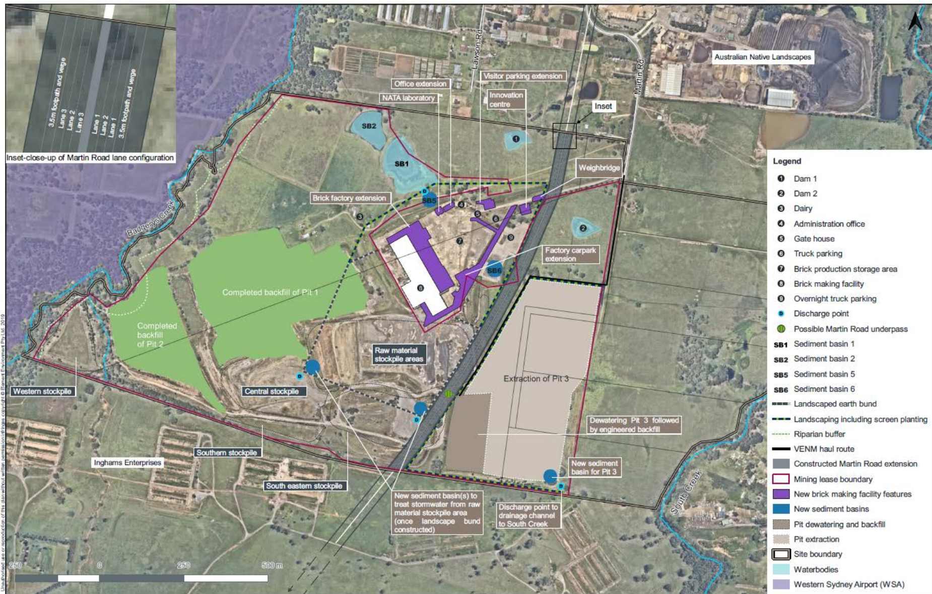
Figure 3: Phase 2 Project Layout
