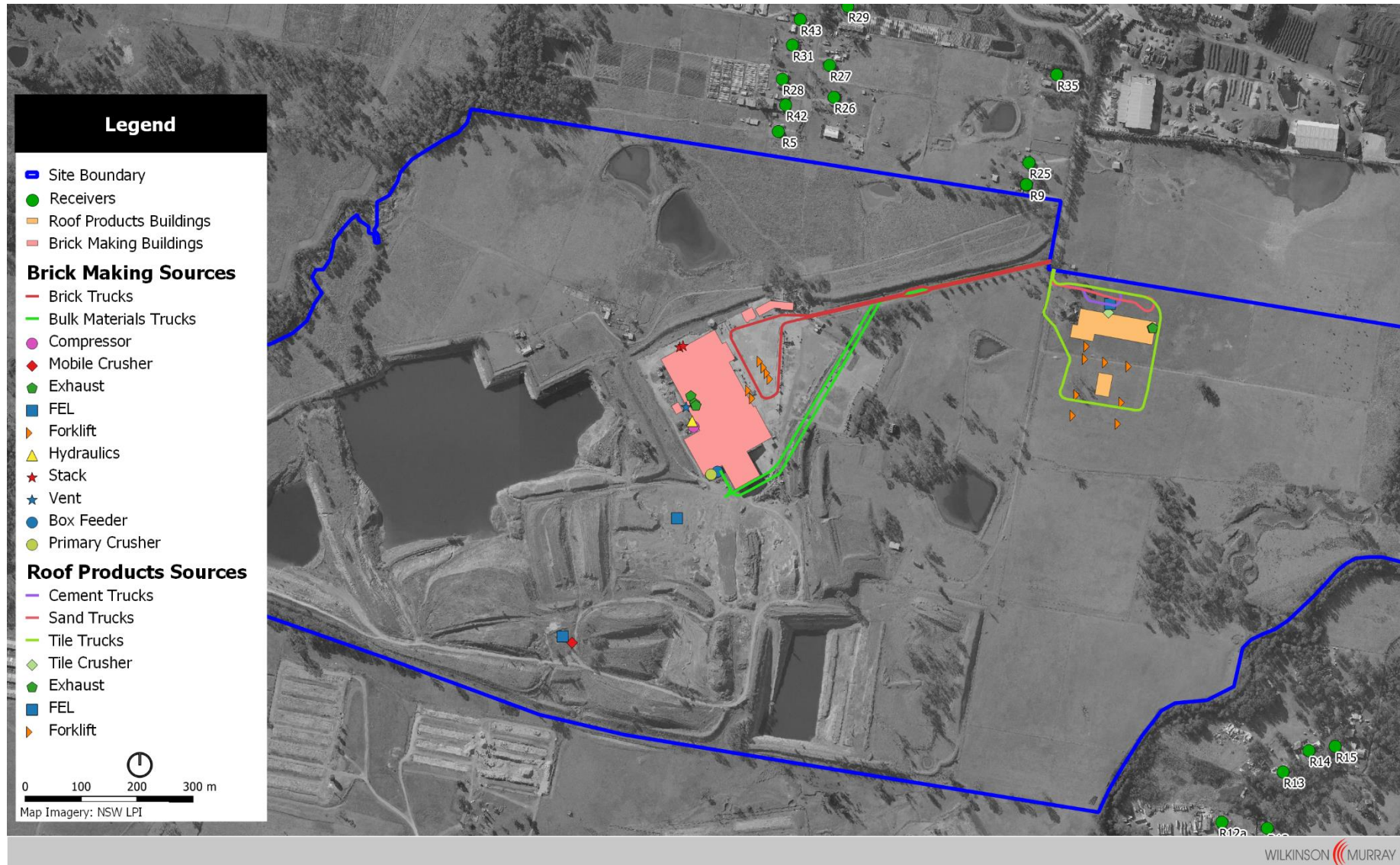
Figure 5-2 Modelled Noise Sources – Brick Making and Roof Products Facilities
