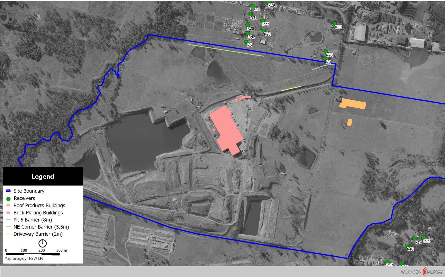
Figure 5-3 Operational Noise Mitigation
