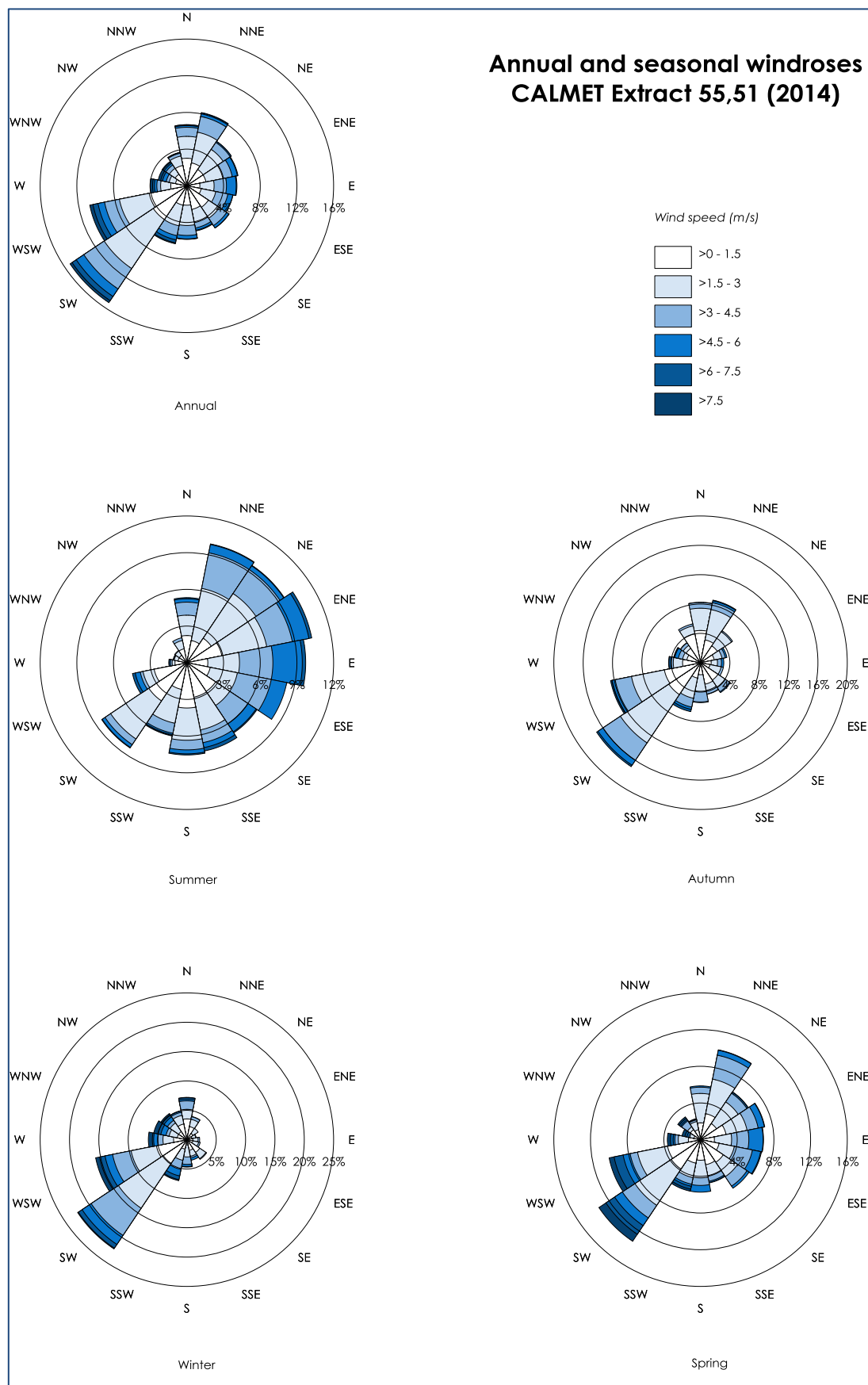
Figure 8-2: Windroses from CALMET extract (cell ref 5551)
