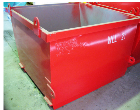
Figure 2B. Contaminated waste bin.
