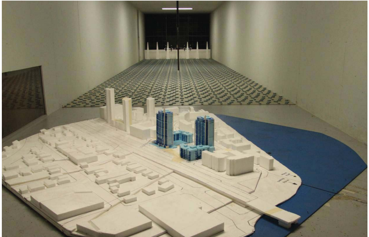
Figure 1c: Photograph of the Wind Tunnel Model (view from the north-east, facing south-west)
