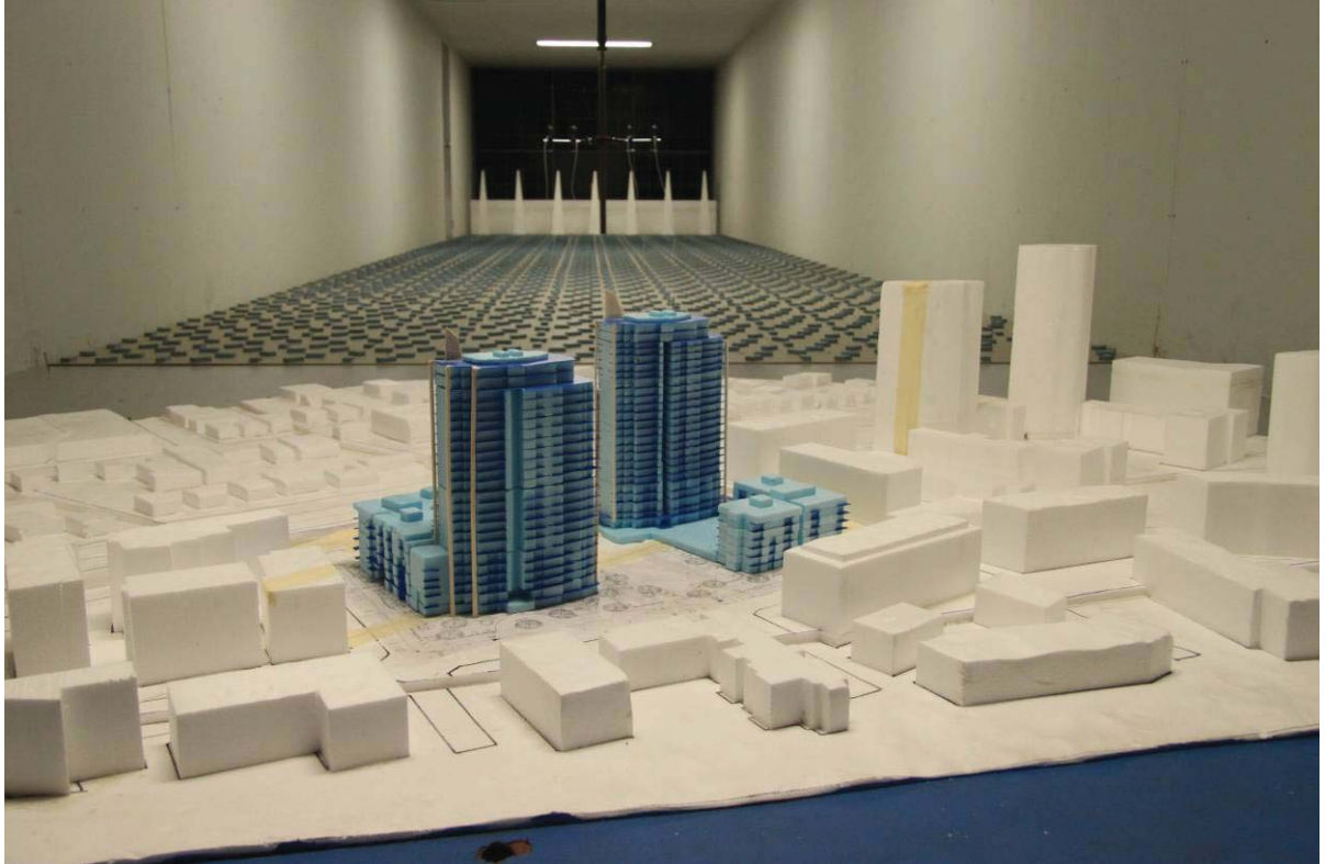
Figure 1f: Photograph of the Wind Tunnel Model (view from the north-west, facing south-east)
