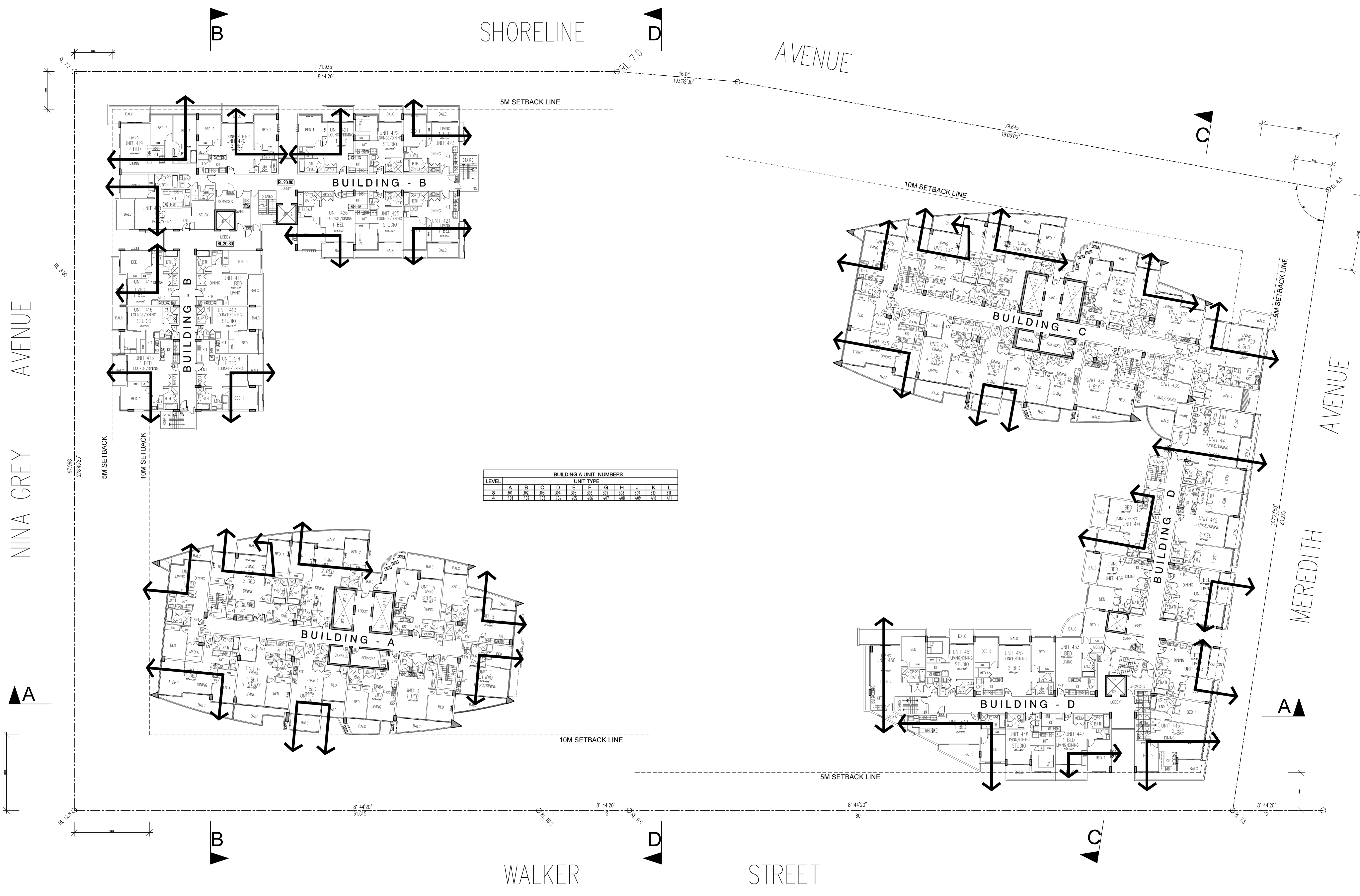
CROSS VENTILATION LEVEL 4 PLAN SCALE 1:200
