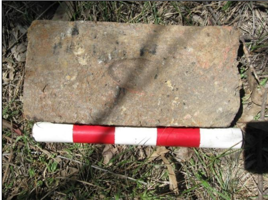
■ Figure 5-24 Intact solid brick with makers mark, probably a convict brick.
