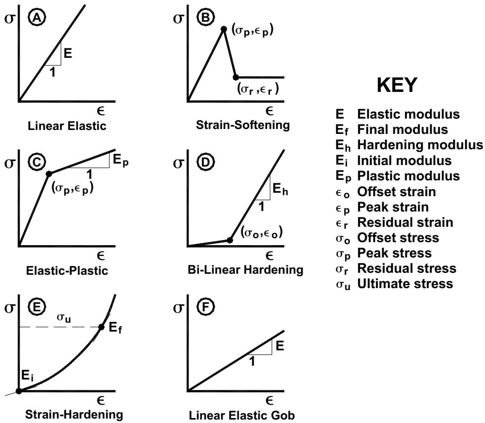
Figure B.1. Stress-Strain Curves for the material models in LaModel and MuSim.
