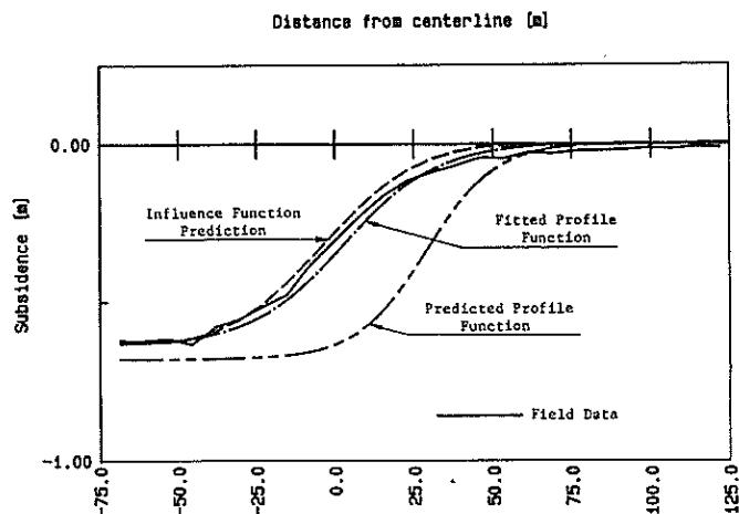
Figure 11 Example #1: Field data and prediction curves
