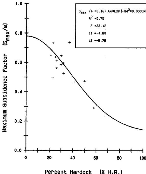
Figure 7 Effect of lithology on maximum subsidence factor
