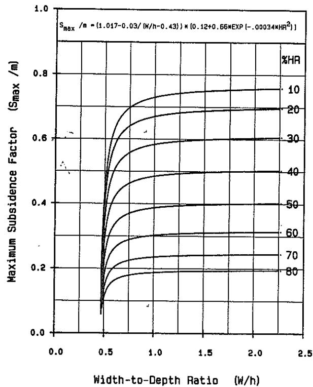
Figure 8 Nomograms for maximum subsidence prediction
