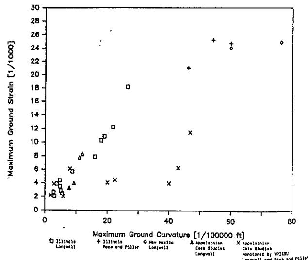
Figure 9 Maximum ground strain and curvature data
