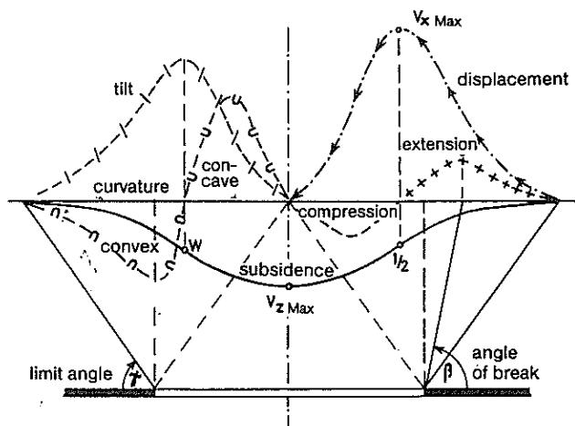
Figure 3 Components of ground movement (after Kratzsch, 1983)
