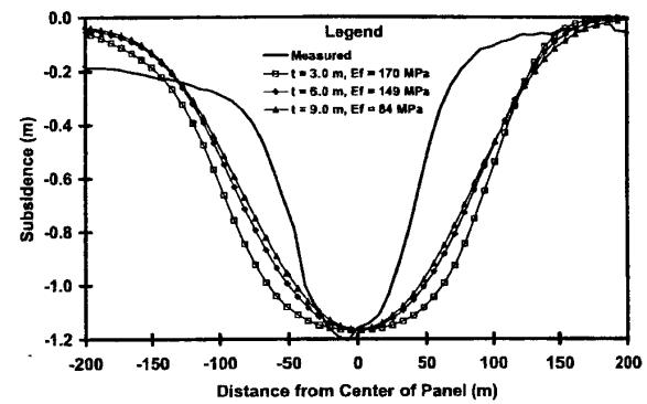
Figure 11 — The measured and fitted subsidence for the E-2 Panel.
