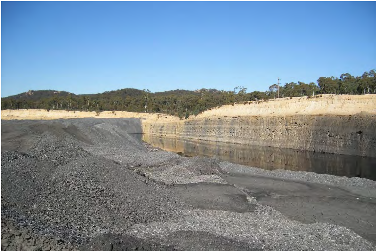
Figure 5 – REA 6, looking South West, showing current deposition level and coarse reject emplacement
