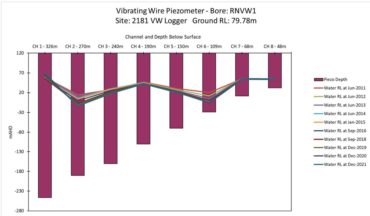
Figure E.3: Vibrating Wire Piezometer - Bore: RNV1 (Site 2181)
