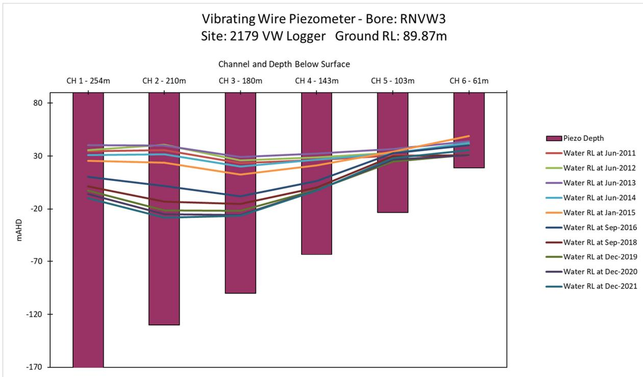
Figure E.5: Vibrating Wire Piezometer - Bore: RNVW3 (Site 2179)
