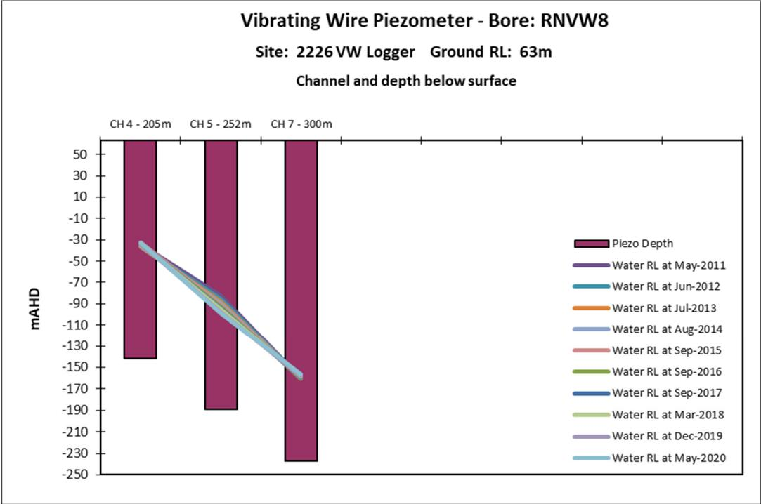
Figure E.10: Vibrating Wire Piezometer - Bore: RNVW8 (Site 2226)
