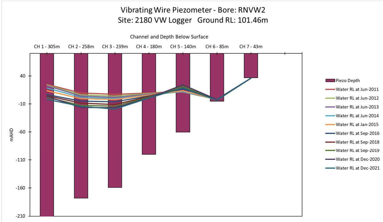
Figure E.4: Vibrating Wire Piezometer - Bore: RNVW2 (Site 2180)
